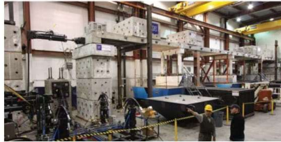
1/4 scaled 33 m long, 4-span bridge
